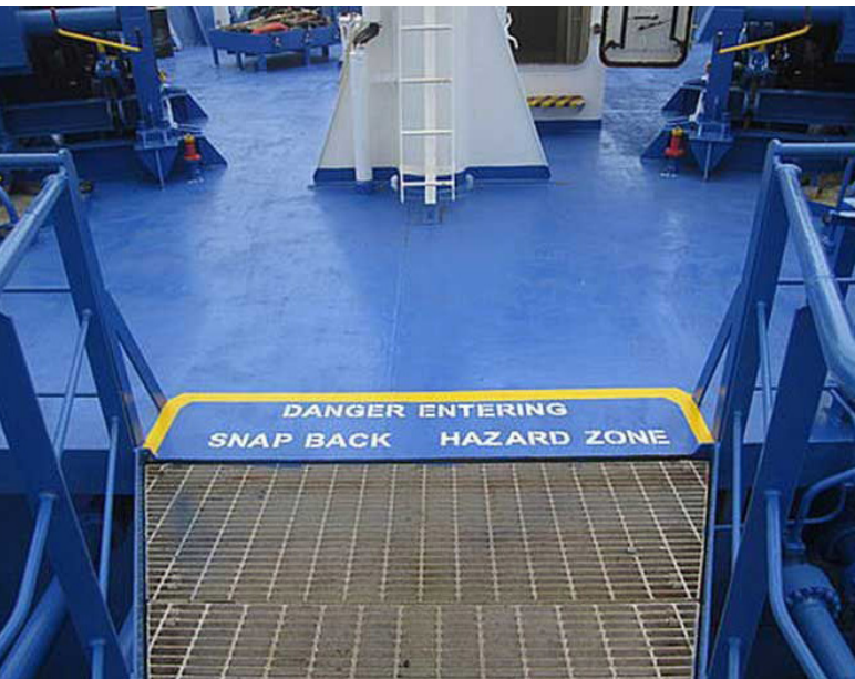
Figure 25: Correct marking for snap-back hazard zone
